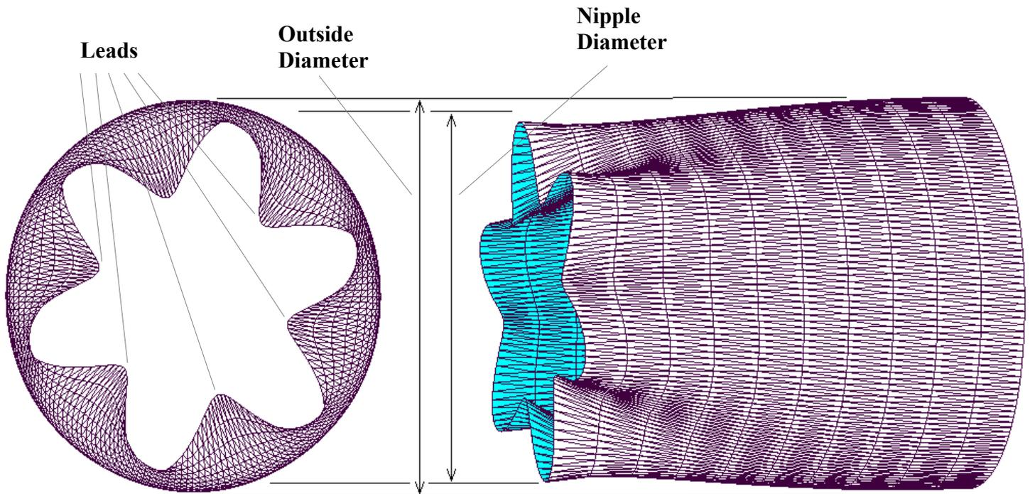
Fig. 1 End view of nipple and outside diameter
