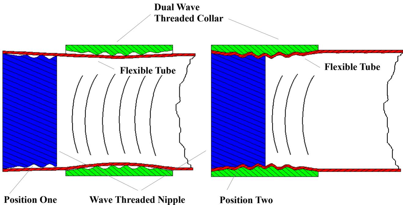
**Fig. 6 Flexible Tube with collar and nipple screwed on**
