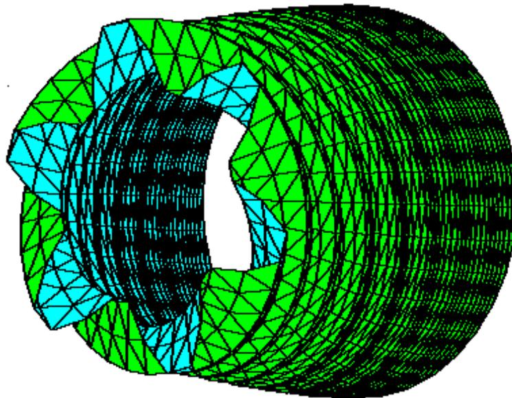
Fig. 5 Angled view of rotated layers forming a wave thread
